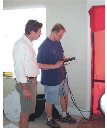
*Energy Rater performs blower door test to measure air tightness.*
